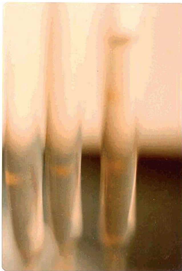
Figure 6. Structures forming from initially homogeneous lead iodide sol in gel (produced by mixing 9 mM KI with 2.25 mM \text{Pb}(\text{NO}_3)_2 in a 0.5% agar–agar solution), on top of which was placed a solution containing KI with concentrations (left to right) of 0.9, 4.5, and 9 mM. Diffusion of the electrolyte occurs out of the gel up into the supernatant solution (from ref 53, Figure 5).
